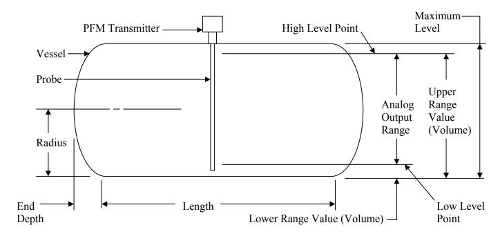
Determine the Maximum Level. This is the highest point that can possibly be measured. This is usually, but not always, the same as the tank height. Fill in the value below.
